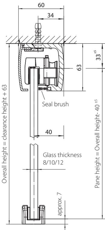
**For fixing to the ceiling with integrated side piece**
